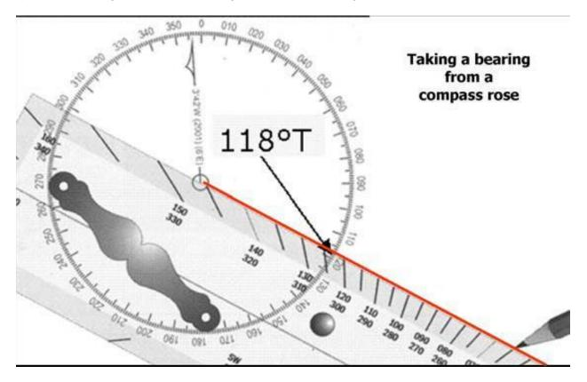
The working chart on the plotting table has a transparent compass rose superimposed and centred over the station's charted position. Now draw a line from the station towards and beyond the anticipated target position.
