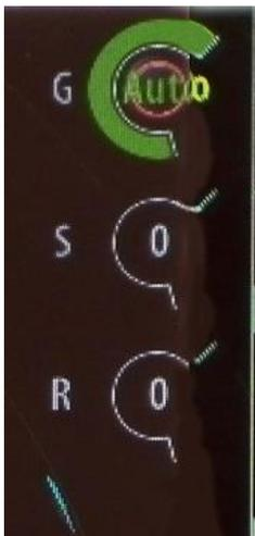
**Receiver Gain** – 2 modes, **Auto gain** is set by the processor to achieve the best picture as determined by prevailing conditions. **Manual Gain** is set by the operator to obtain best picture – ***Beware if conditions change the radar gain remains the same.***
