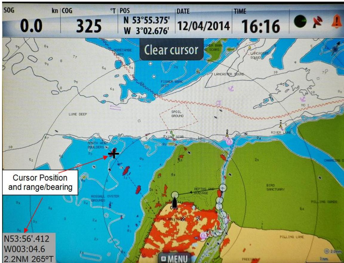
On this display, the radar contacts are shown in Red and note they are transparent showing the chart beneath.
